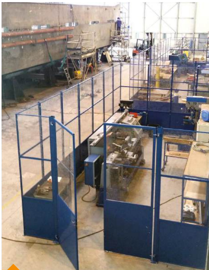
Integration of a 5S partition to make a safe working area and protect it against draughts.
